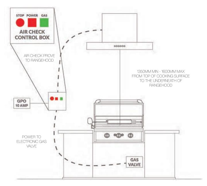
Capital's Air Check is a self-contained device designed for Commercian and indoor BBQ installations, where there is a requirement for the appliance to have an interlock installed. The Interlock system is designed to only allow the Gas Valve to open once, the extraction fan is operating. Once the rangehood is operating, gas will flow to the appliance and the BBQ can be ignited. Ref: AS/NZS 5601.1:2013 Clause 6.10.1.15
